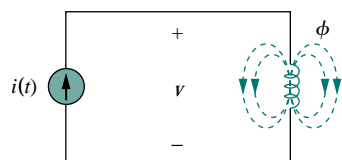
Figure 13.1 Magnetic flux produced by a single coil with N turns.
